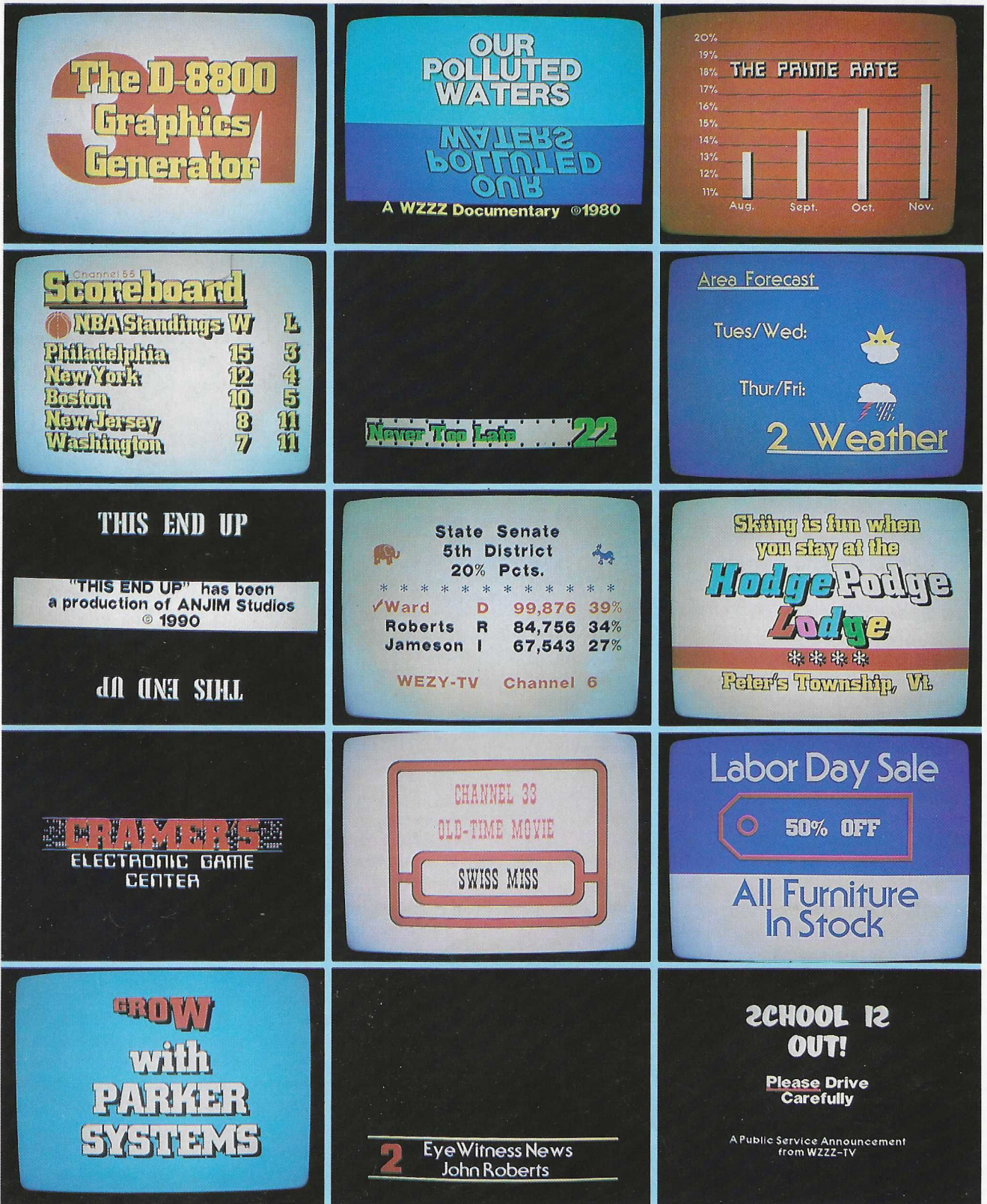
The above are typical displays utilizing D-8800 features; such as, dual channel mix, mirror image, character invert, character reverse, logos, left and right italicize and line segment font. All displays are created directly from the D-8800 keyboard.
