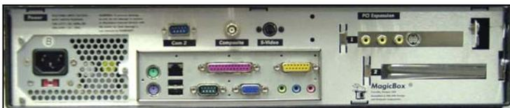
The back panel has a variety of connections for attaching various monitors and accessories to the unit. These connectors are described later in this manual.
