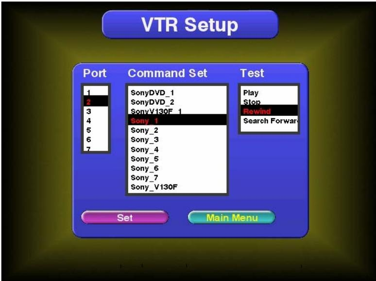
1) Select the Port. The port is defined by the output Infra-Red emitter that is affixed to the face of the VTR/DVD unit. Use the Right arrow to move to the Command Set panel.
