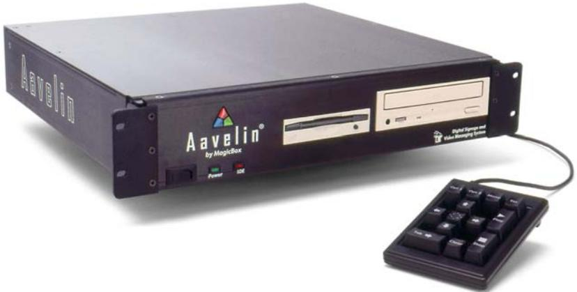
The Avelin Digital Signage and Video Messaging system allows you to create slides and other content on your PC with graphics and text which can then be played back on numerous types of video monitors using the Avelin unit.
