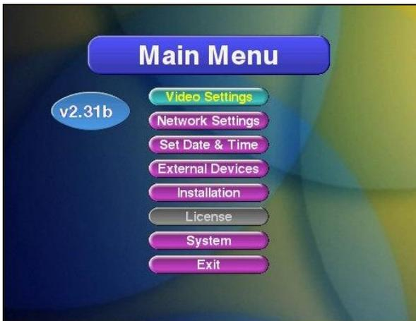
The Aavelin’s menus are sent to all video output connectors simultaneously: VGA, Composite, and S-Video, at a resolution of 640x480. This allows the menu to be viewed regardless of what kind of monitor is connected.
