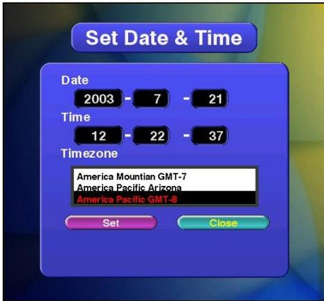
Use the left and right arrow (← →) buttons to select the field you wish to modify, and use the up and down arrow (↑ ↓) buttons to change the value of that digit. Press Select (⊠) to move to the Time line, and follow the same procedure to set the values there.
