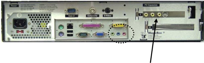
The default video input connector is Composite Input 1 (see arrow).
