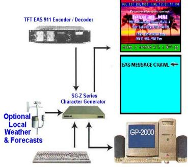
The EAS 911 Alert System shown above illustrates the use of a single character generator system used for a community bulletin board to now also provide the required EAS Alert without the purchase of an additional character generator.
